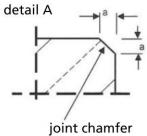
a = chamfer face (3 to 10 mm)
